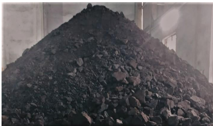
Fig. 2: Composite sample: blending of five different seam samples in equal proportion.
