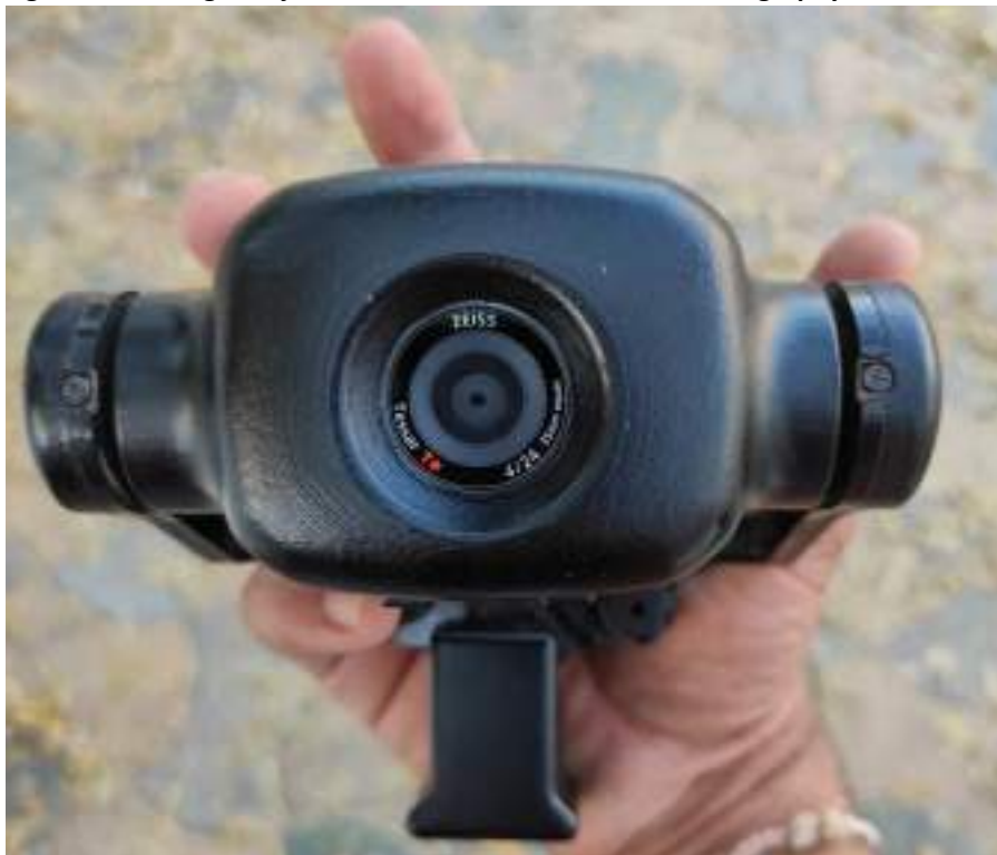
Fig 3.3.7 High Resolution 20 mp Sony camera used in Drone photography
