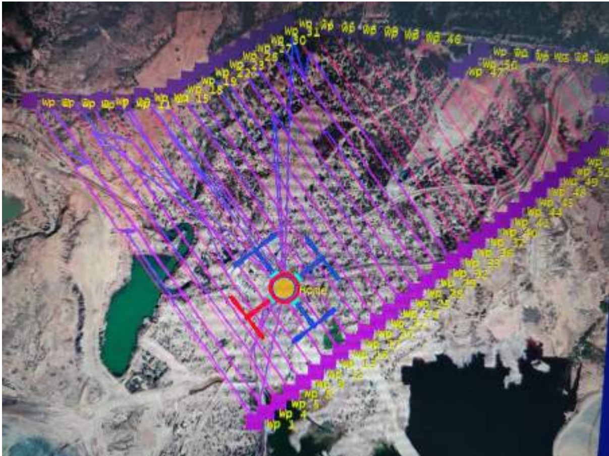
Fig 3.3.8 Flight plan for Drone Photography
